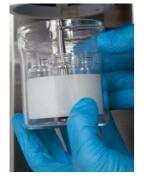
miVac SpeedTrap is supplied with a one litre glass condensing vessel.
